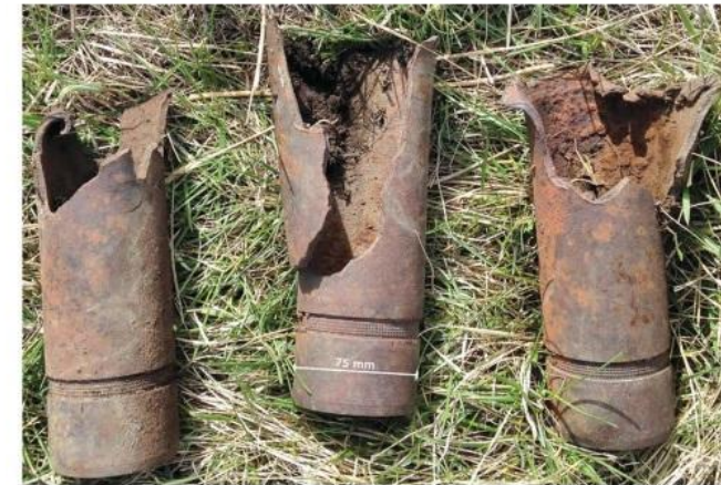
75mm shrapnel projectile munitions debris recovered from north slopes of Green Mountain in 2014 as part of the Camp George West Remedial Investigation.
